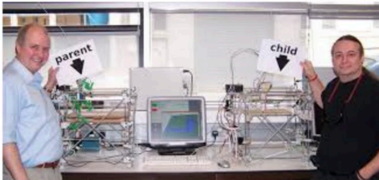
fig. 3: RepRap self-replicating 3D printer with original and copy.
